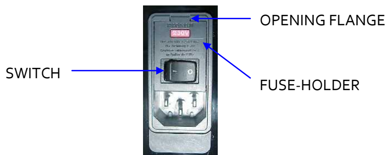
Figure 1. Power inlet, main switch and fuse holder.
